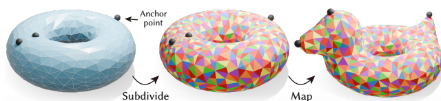
Figure 25: Our method allows base meshes with different shapes but with the same topology.
