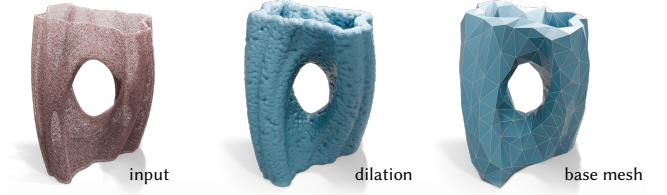
Figure 16: On a non-oriented point cloud where the occupancy function is unavailable, one may dilate the points for a certain radius by adding an offset to the distance function on a regular grid.
